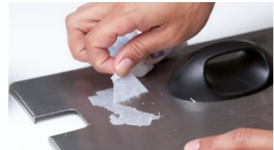
Figure 4: Depiction of a substrate failure [26]. The substrate fractures during the peel such that <100% of the substrate is removed leaving both adhesive and substrate residue behind on the surface
