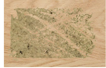
Figure 3: Depiction of a cohesive failure [25]. 100% of the substrate and <100% of the adhesive is removed from the bulk material surface, with the remainder being left behind as residue on the surface.
